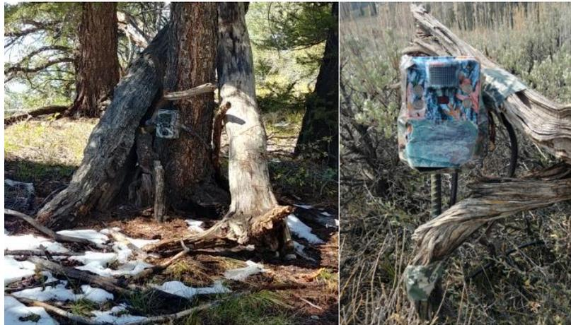
Figure 2. Tree set up of a Reconyx on-trail camera (left) and a sagebrush post set up of a Browning on-trail camera (right).
